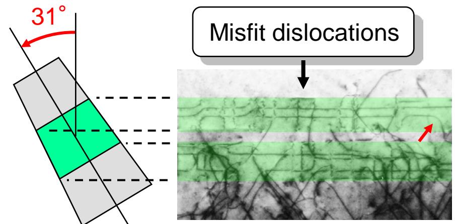
Threading dislocations can change into a misfit dislocation at interfaces.
