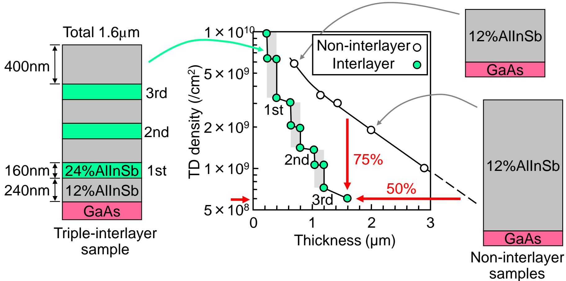
$\text{Al}_x\text{In}_{1-x}\text{Sb}/\text{Al}_y\text{In}_{1-y}\text{Sb}$  interlayers can be used to improve the performance of any InSb- (InAsSb)-based devices in which  $\text{Al}_x\text{In}_{1-x}\text{Sb}$  is used as a buffer, insulating, or barrier layer material.
