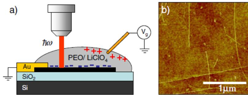
FIG. 1 (color online). (a) Schematic diagram of the experimental setup. The excitation laser shines through the PEO/LiClO<sub>4</sub> polymer electrolyte. (b) An AFM image indicating that the nanotubes are spaced out and are typically isolated from one another.
