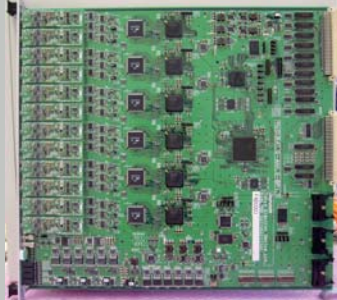
Front End FPGA: Spartan 3E x 6 System FPGA: Spartan 3 x 1 User FPGA: Virtex 2 Pro x 1
