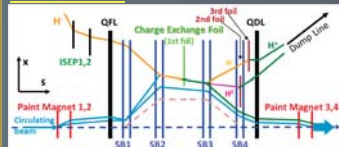
Fig : The schematic drawing of Painting Injection and phase space at 1 st Foil
